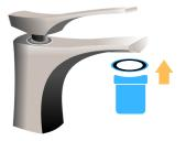
For Taps with F24(Inner) Threads, Place the Washer above the Nozzle and insert into the Tap.
